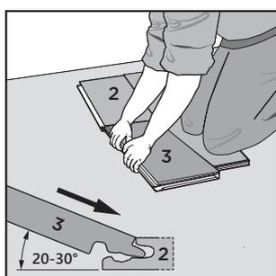
Angle in the short side of panel 3 into the short side of panel 2 at 20-30° and angle down.
