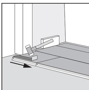
For edge pieces close to the wall, use the pull bar and hammer to completely secure the locking system. Gradually connect the panels in a few taps.
