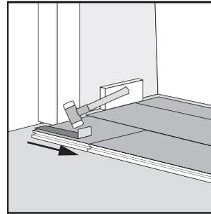
Slide the panel towards the already installed panels and gradually lock the short side of the panel with a tapping block or pull bar and hammer in a few taps.
