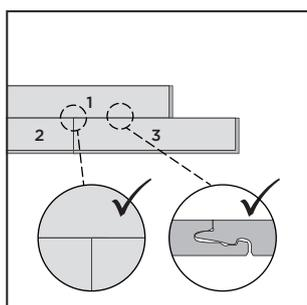
After installing a panel, check if all joints are fully connected and there are no gaps or height differences.
