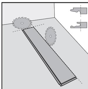
Remove the click profile on every side directly next to the wall to ensure the required expansion gap.
