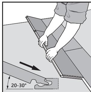
Place your hands close to the joint and move the panel up to an angle of 20-30°. Pull the panel towards the installed panels and angle down.
