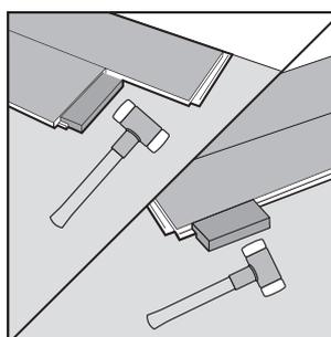
To ensure all gaps are closed, gently tap the tapping block with a hammer to completely close the joints.
