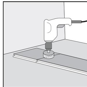
Click the panels together on the short side. Drill a hole centered on the joint between the two panels of the same diameter as the pipe plus 20 mm (3/4").
