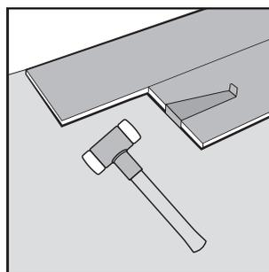
Use a pull bar and position it against the locking system. Gently tap the pull bar with a hammer to gradually connect the panels in a few taps.
