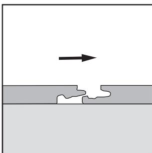
For areas where it is not possible to use angling or a tapping block, such as the end panels against the wall, use the pull bar with the tapping method.
