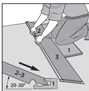
Place your hands close to the joint and slide panel 3 towards panel 1. Angle the row of panel 2 and 3 up to an angle of 20-30°. Angle down to completely connect the panels.
