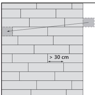
Tip: use the leftover of the sawed off panel to start the new row. Stagger the panels randomly and use an overlap of at least 30 cm to ensure a strong connection.
